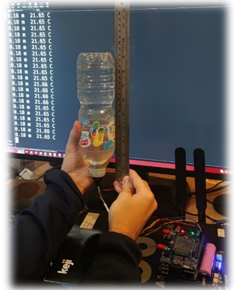
Figure 15: Bar02 Sensor Bench Testing
