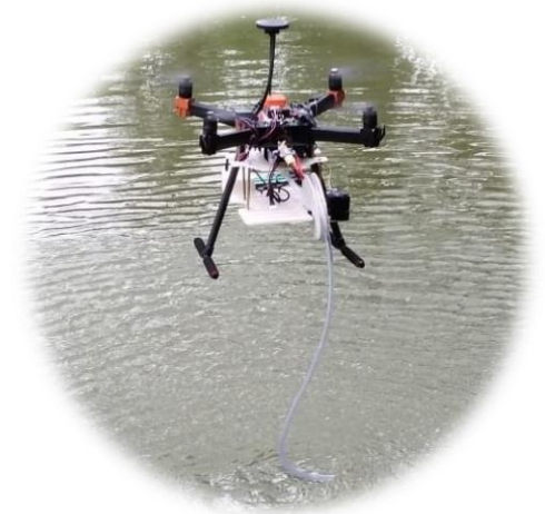
Figure 2: Autonomous UAV Based Water Sampling
