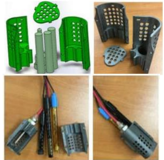
Figure 5: OSMM Custom built multi-Probe
